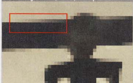
8x MS + Edge-Detect (Radeon): 8 Samples + ED-Filter
