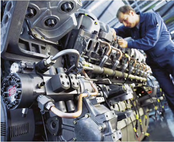
FIGURE 8.19 L'Orange CR fuel injection system installed on an MTU Series 4000 high-speed engine, showing the engine-driven HP pumps feeding the CR and injector pipes
