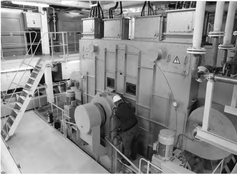
FIGURE 6.5 One of two 15 000 kW STN Atlas propulsion motors installed on the cruise liner Costa Victoria
