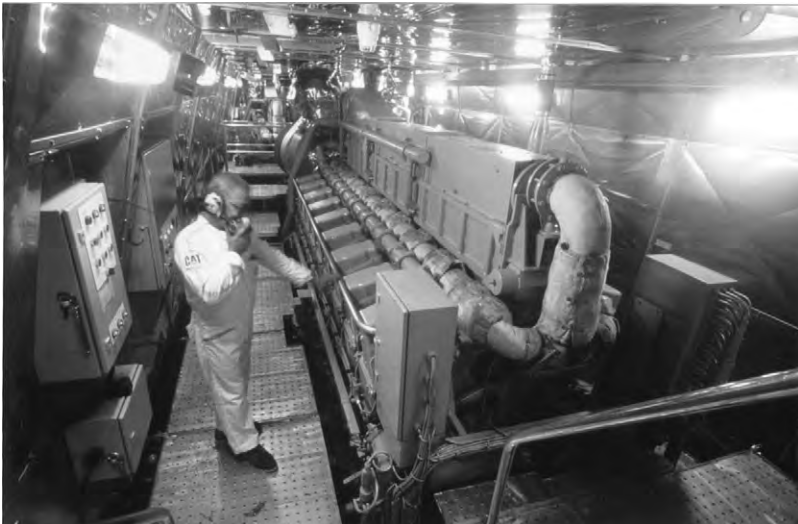
FIGURE 19.3 One of four 7200 kW Caterpillar 3618 engines installed in a fast catamaran ferry
