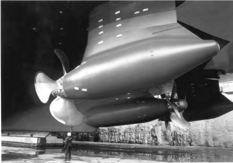
FIGURE 6.8 Three 14 000 kW Azipod propulsors power Royal Caribbean Cruises' Voyager-class liners
